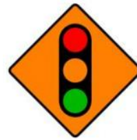
WK 060 - Temporary Traffic Signals
